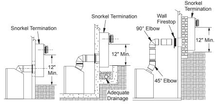
Figure 16 - Snorkel Termination Configurations for Below Ground Installation
